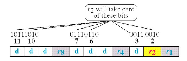
Redundancy bits calculation
