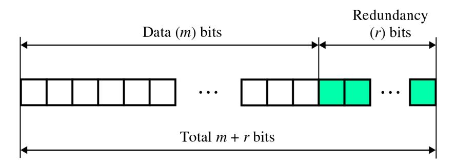
If the total number of bits in a transmittable unit is m+r, then r must be able to indicate at least m+r+1 different states
