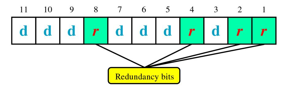
each r bit is the VRC bit for one combination of data bits
