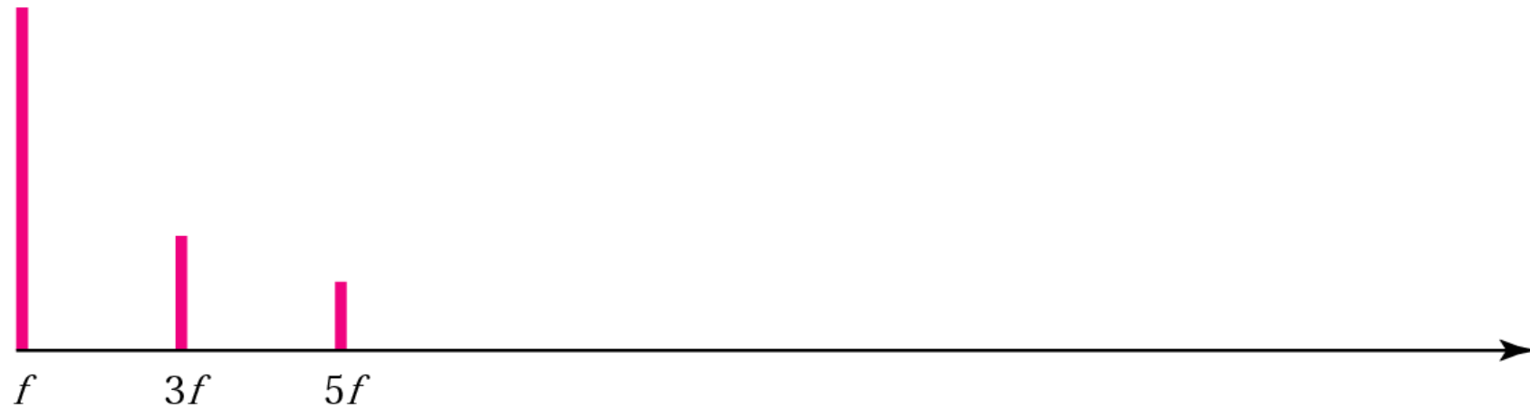
a. Frequency spectrum of a square wave
