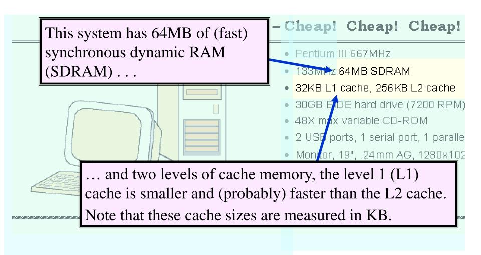
Hard disk capacity determines iter - Cheap! Cheap! Cheap! the amount of data and size of Pentium III 667MHz programs you can store. 133MHz 64MB SDRAM 32KB L1 cache, 256KB L2 cache 30GB EIDE hard drive (7200 RPM) 48X max variable CD-ROM 2 USB ports, 1 serial port, 1 parallel po This one can store 30GB. 7200 RPM is the rotational speed of the disk. Generally, the faster a disk rotates, the faster it can deliver data to RAM. (There are many other factors involved.)
